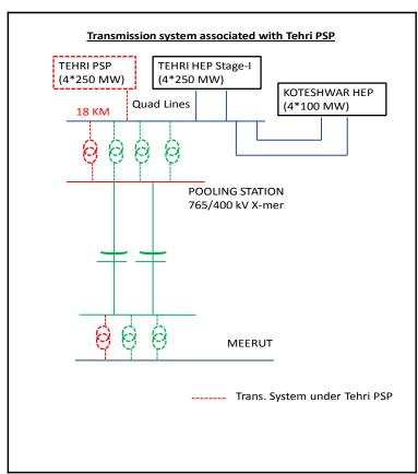
CTU stated that with 1400 MW installed capacity at Tehri complex, three 800 MVA ICTs would be sufficient for meeting the n-1 criteria; therefore they have proposed the charging of 3x800 MVA ICTs. He added that at present all the three ICTs have been charged along with the charging of Tehri-Meerut line at 765 kV level.
